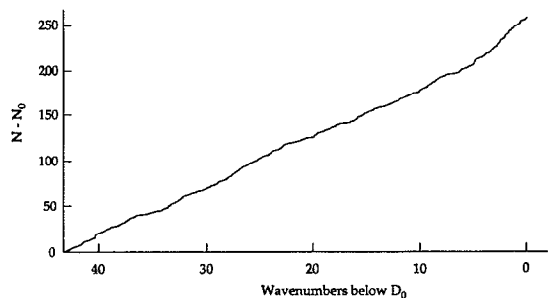
FIG. 8. Number of observed transitions vs energy, relative to D_0 - 45 \text{ cm}^{-1} . The transitions are from the spectrum shown in Fig. 6.
